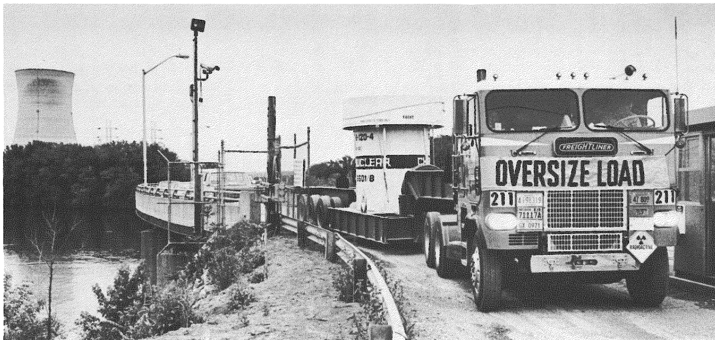
PF-16 liner leaving TMI for characterization at Battelle Columbus Labs. (GPU Nuclear Photo)
