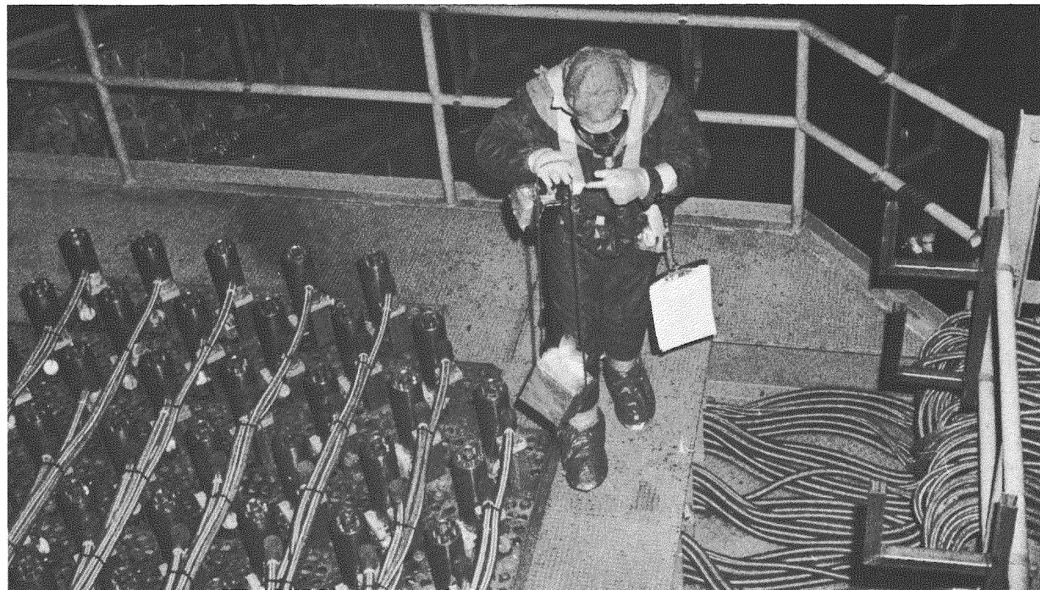
Physics technician performing the first radiation survey on the top of the control rod drive mechanism service structure. (TIO Photo Entry 7)
